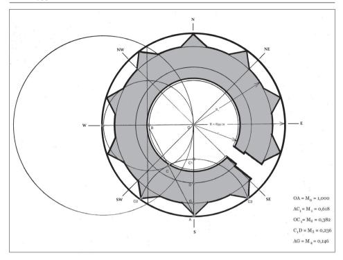
Figure 4. Oriented plan of the Gonbad-e Kāvus tower with indication of the parts ( $M_0, M_1 ...$ ), given R = 1
